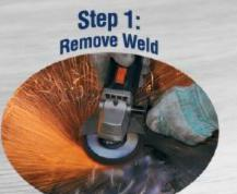
Circular Scratch Pattern - Grind weld down with a 24 - 40 grit aluminum oxide, zirconia, or ceramic: Flap Disc, Mini Flap Disc, TWINPOWER, Coated OC Disc, Fiber Disc
